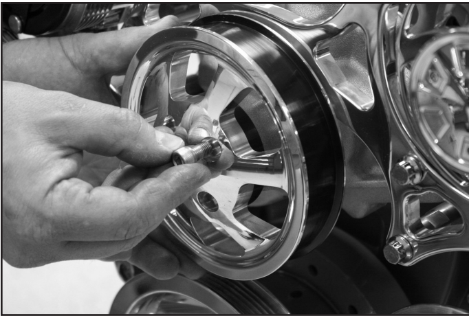
Figure 12: Install Water Pump Pulley
